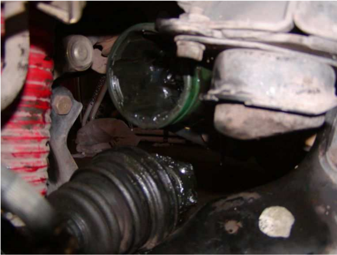
Next you pull the CV joint out by pulling the brake assembly outward. This is the result.
