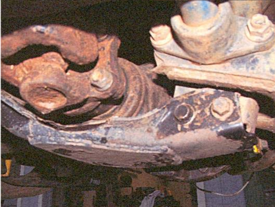
A radius was cut out of the edge of the transmission /exhaust skid plate to clear the driveshaft.
